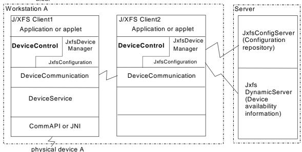
Why is it required that the J/XFS client2 has no local device access? Because it is impossible that multiple Device Services for the same physical device are started. And why that? Because access to the device through the physical port it is connected to is restricted to 1 process only.
