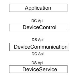
It implements the Device Service interface for the Device Controls to use. For the DeviceService it implements the same interface as the Device Controls do -- which is mainly the IJxfsEventNotification - interface.
