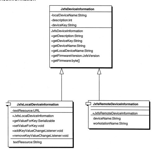
The basic configuration data describing the device is stored in the JxfsDeviceInformation object or in its subclasses JxfsLocalDeviceInformation and JxfsRemoteDeviceInformation. The objects of this classes are a kind of information container hiding configuration structure from the Controls and Services layer; the means how this information is stored / gathered can be changed by different implementations without affecting Device Service and Device Controls.
