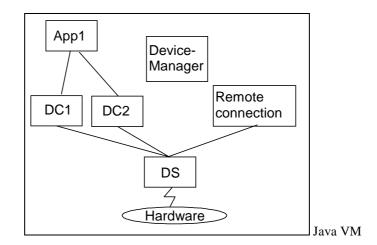
If an application or applet wants to gain exclusive access to a device, it uses the claim() method on its Device Control. The basis is the control object, i.e. that if an application gets two control objects for the same device a claim() to the second one will fail, even though it is used by the same application. So, an application can either use one control for all its activities with a device or use the claiming mechanism to synchronize its different program parts if necessary.
