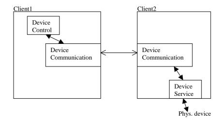
The above chart tries to give a short sketch of how the communication classes enable the sharing of devices across a network.
