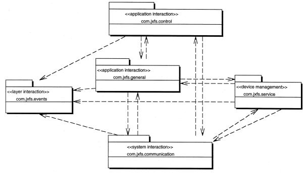
The lines represent dependencies between the different packages. The most important concept here is that the Device Service layer does not depend on the Device Control layer as only then can the chore of transferring data over a network be invisible to the Device Service as well as to the application.
