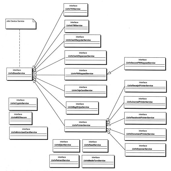
The diagram depicts the inheritance tree of the device service interface classes. Also shown are some of the available mixin interfaces to add special functionality (e.g. the support for motorized card interface for the MagStripe and ChipCard devices). These are the ones which do not inherit from the IJxfsBaseService interface.
