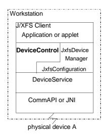
The application requests the device from the DeviceManager and accesses the device via the DeviceControl. The DeviceControl is directly connected to the DeviceService for the device. The JxfsDeviceManager controls both objects. The whole configuration may be kept locally, either hard-coded in JxfsConfiguration object or somehow configurable on disk or in memory.
