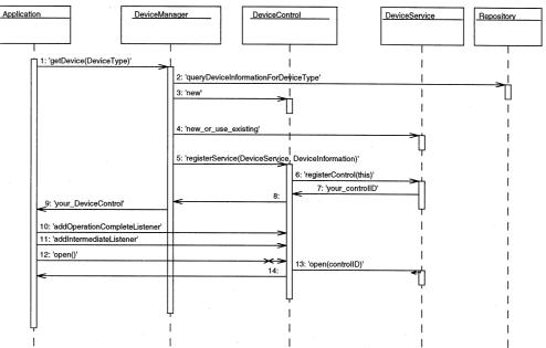
• **IJxfsBaseControl getDevice(Class control\_classname) throws JxfsException;** Here, the application requests a device of type control\_classname without specifying a concrete name. The DM should return a Device Control for the default device of this type for this J/XFS client or - if no default is configured - to the first such device found. If the application stops using the device it must be released and then deregistered with deregisterDevice().
