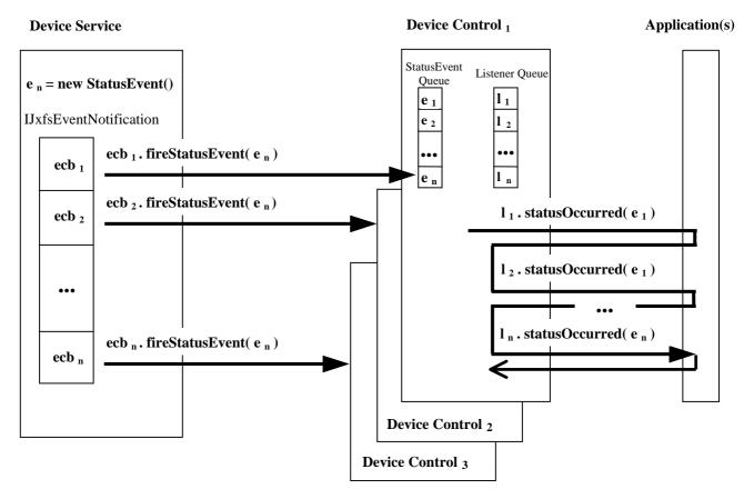
Each thick black arrow represents one thread. The Device Service generates an event and delivers it to every Device Control it is connected to (Shown here are three DC's). The threads only add the new event to the respective queue in the Device Control and immediately return to the DS. Now a separate thread running in the DC always picks the next available event in the queue and delivers it to all application objects which have
